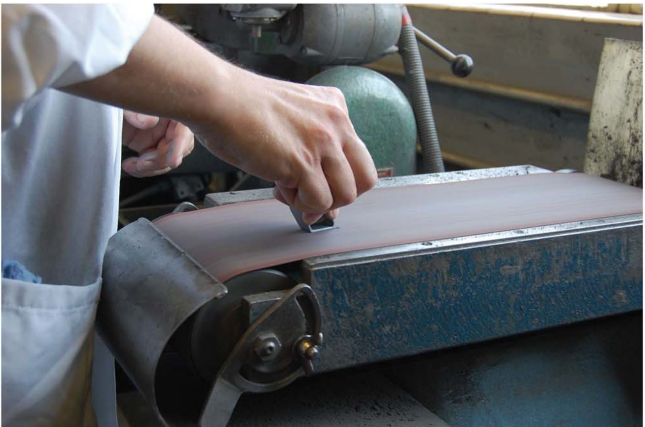
Putting a slight angle on the tonearm counterweight-this move is almost imperceptible to the eye. Too much pressure for a second too long means the trash heap.
