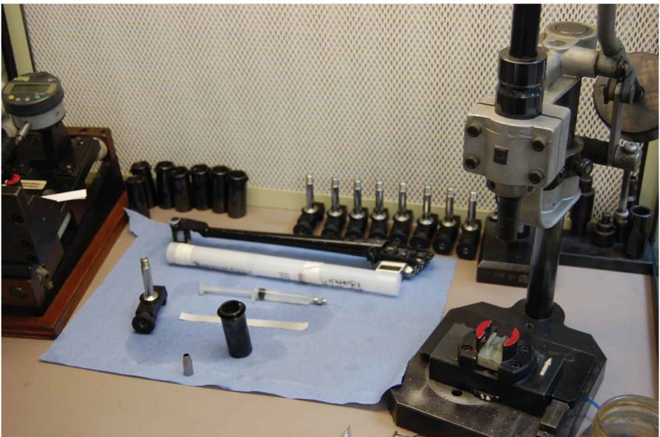
This is the work station for the critical vertical bearing assembly; the small hand press (right) is used to check tolerances/resistance.
