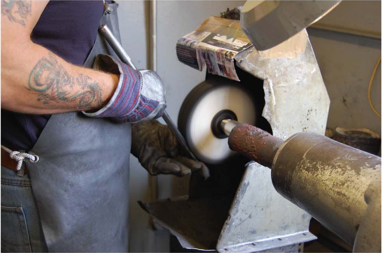
Putting a bit of muscle into polishing a stainless steel armtube for the M2-9 tonearm
