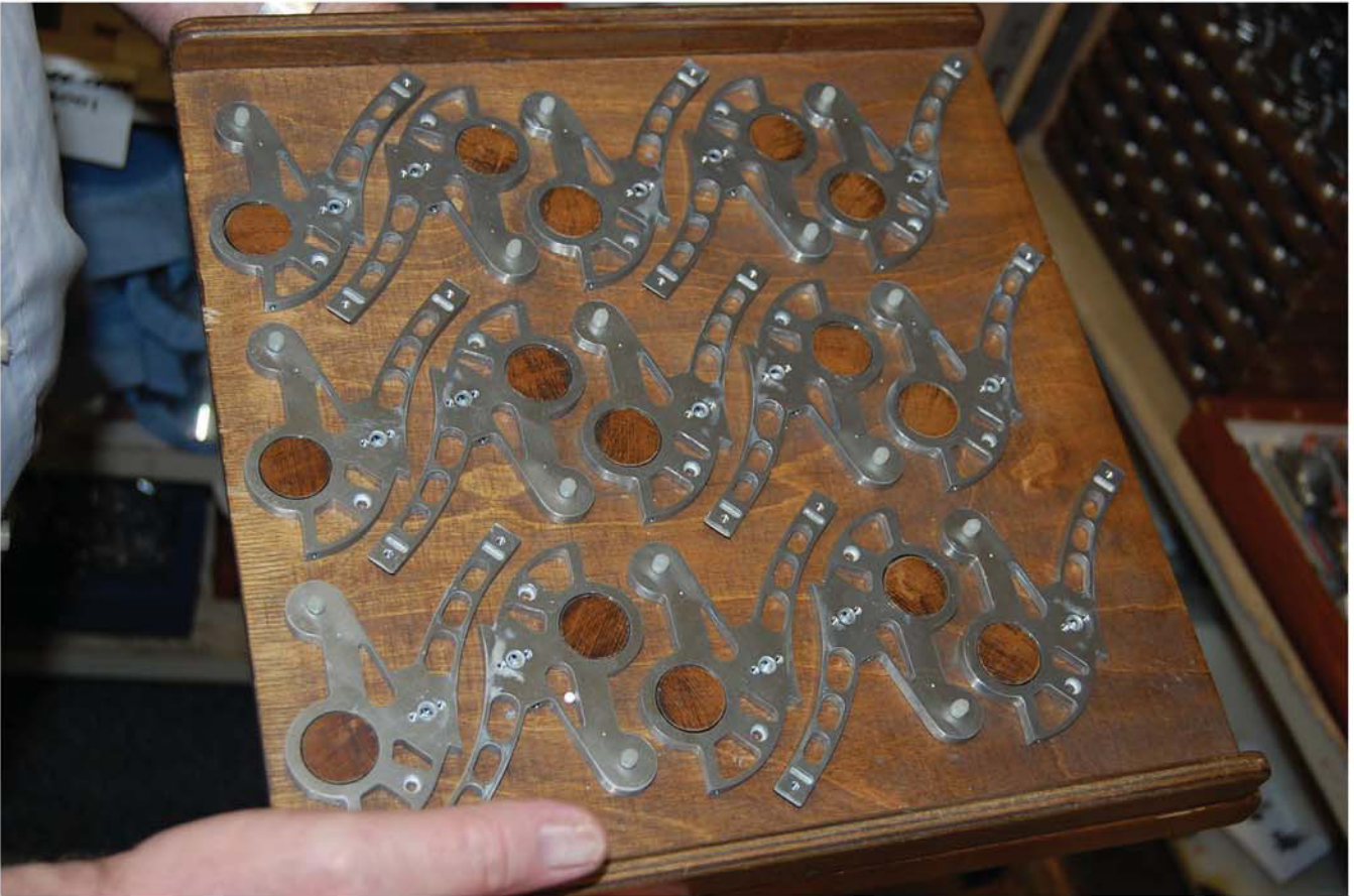
Control arm brackets drilled and tapped prior to final machining, Placement on the jig keeps them from damaging each other.
