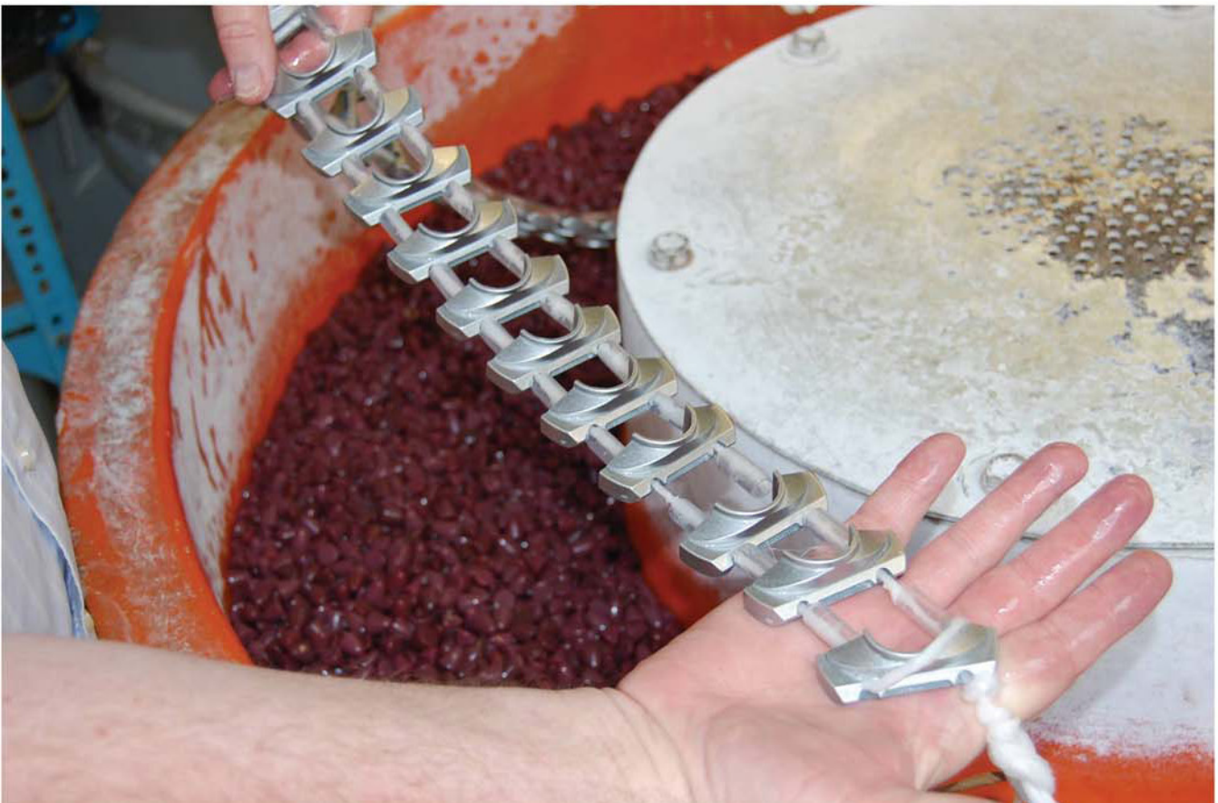
The rumbling or barrelling machines and plating. Different grades and sizes of these resin pebbles act like very fine sandpaper to gently round every hard edge. Usually runs about eight hours, generally through the night.
