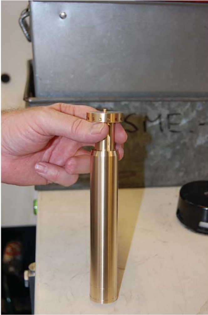
A gorgeously finished top gallery suspension column for SME 30- followed by the raw, rod material that begins the process.
