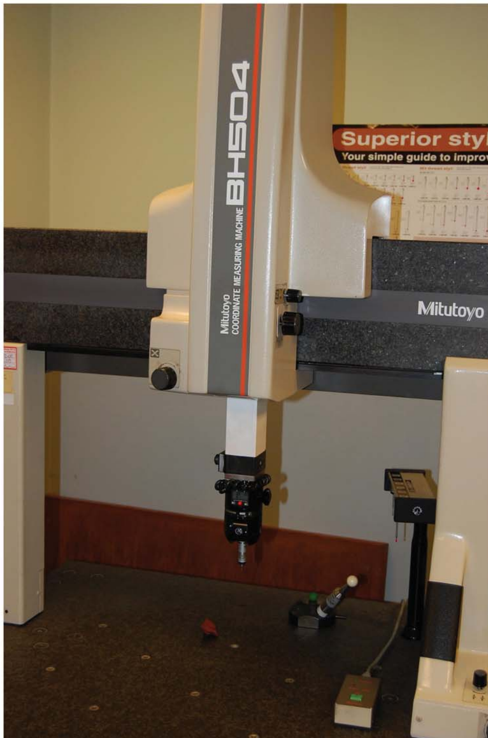
A CMM or coordinate measuring machine CMM that is programmed to check a part's dimensions for accuracy and flatness relative to itself and other impacted parts
